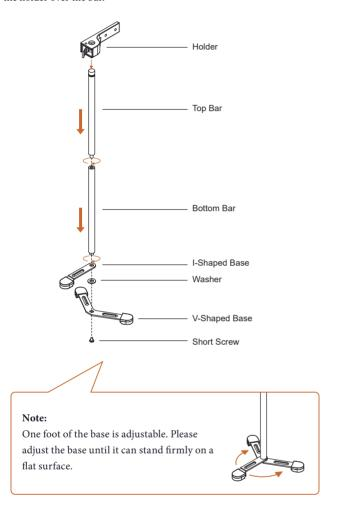
2. Slide the holders up and down to adjust the position and height to match various GPU cards and PC cases.
