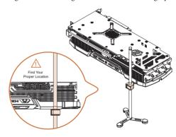
Attention! The illustration is for reference only. Please find a proper location, based on the graphics card you have, for the holder, and make sure the holder will not interfere with the GPU fans and PCIe power connector(s).
